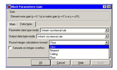
The four fixed-point Simulink rounding modes are discussed below. The data is generated using the Simulink Signal Generator block, and doubles are converted to signed 8-bit numbers with binary point-only scaling of 2<sup>-2</sup>.
